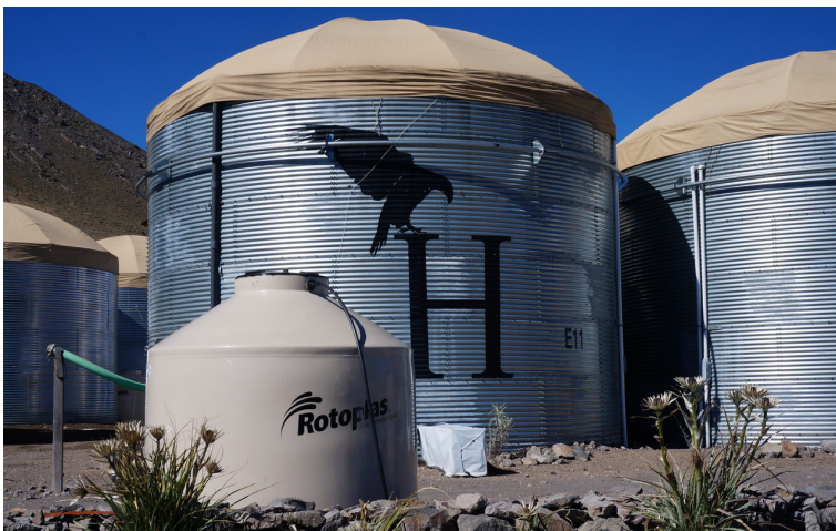
One of the ‘outrigger’ tanks in front of the main detector array of HAWC in Mexico.
